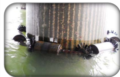
MGP-W SC protecting a new pile from marine growth settlement
