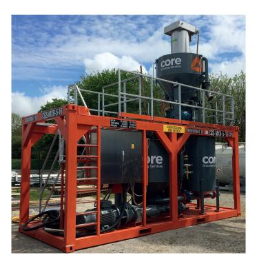
Continuous mixing and pumping unit for large volume grout applications. Housed in one (1) DNV certified frame for ease of mobilisation.
