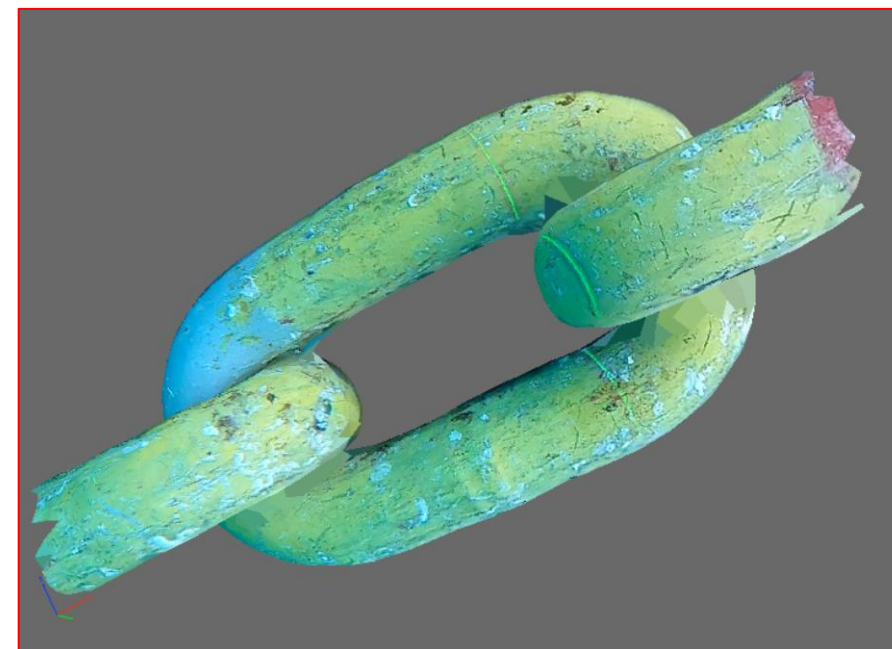
Mooring Chain Measurable 3D Model
